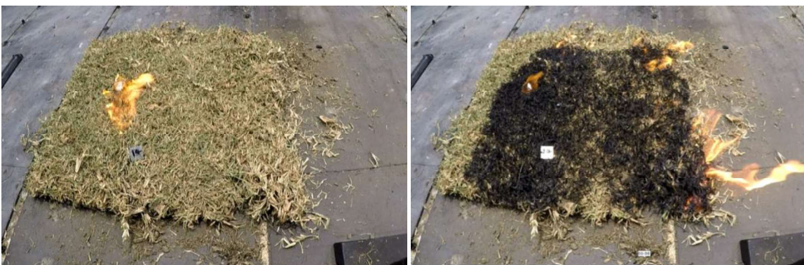
Figure 8 Sustaining ignition in buffalo grass turf with a strong wind speed (ignition number 167). Unburnt fuel is visible underneath the burnt tips (right)
