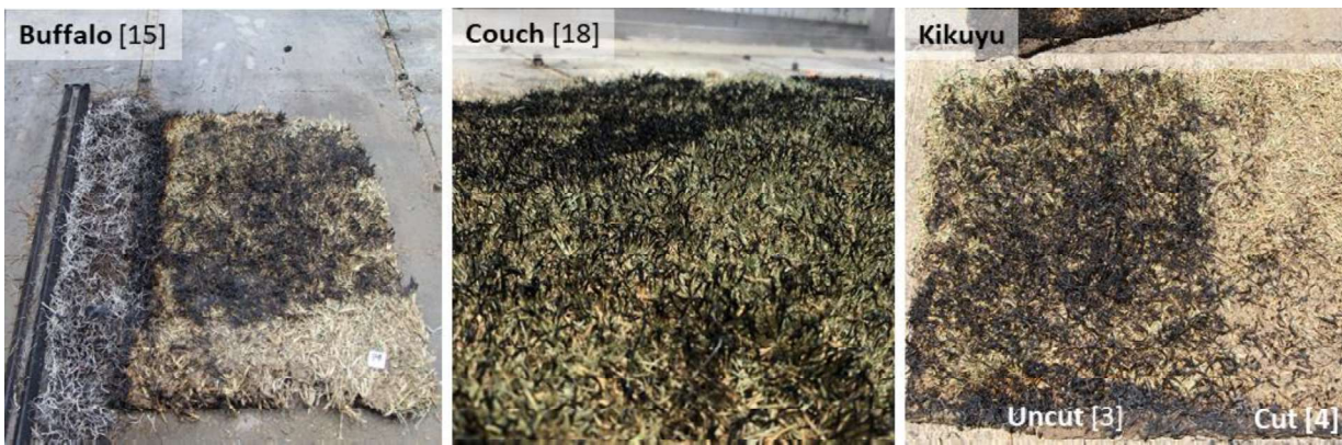
Figure 17 Post fire images showing residual charred fuels following spread sustainability tests for the different turf varieties. The numbers refer to the fire reference, see Table 5.
