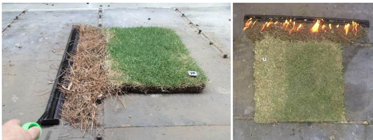
Figure 6 The experimental setup used for line fire spread sustainability tests showing the side view prior to pilot ignition (couch) and the plan view immediately following ignition (kikuyu, cut and uncut).
