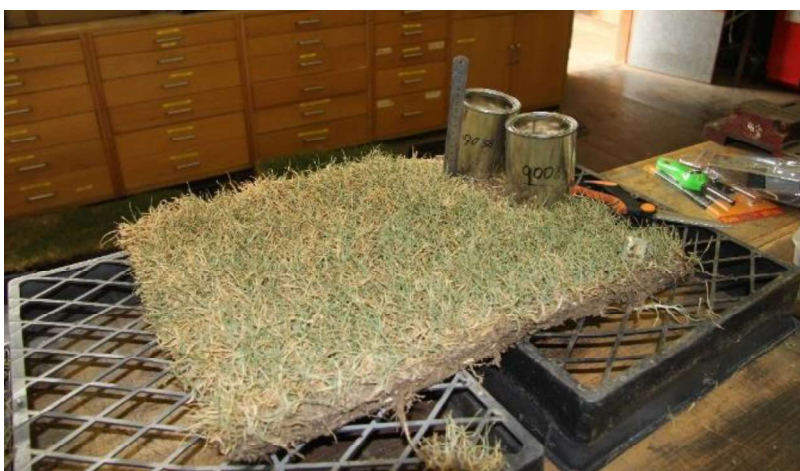
Figure 2 Cut turf samples being dried on an aerated base prior to experimentation.
